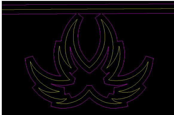
Chamfer corner type; offset Both sides 0.2".
